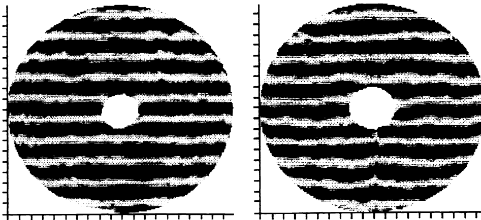
FIGURE 3. Synthetic interferograms of the finished primary (left) and secondary mirrors (obtained from averages of 15 phase maps). The 1.8-m f/1.0 ellipsoidal primary mirror was stressed-lap polished at Steward Observatory to a surface error of 17-nm rms and 170-nm p-v. The Strehl ratio is 90% at 633-nm. The phase maps were obtained with a Shack cube interferometer and refractive null corrector. The 0.38-m f/0.9 concave ellipsoidal secondary mirror was polished at Space Optics Research Labs. The final figure was measured at the Steward Observatory to be 13-nm rms and 150-nm p-v surface error with a Strehl ratio of 98.5% at 633-nm. The phase maps of the secondary mirror were obtained with a double-pass interferometer having a Shack cube at one focus of the ellipse and a precision ball bearing reflector at the other focus (the vertical feature is the rod holding the bearing).
