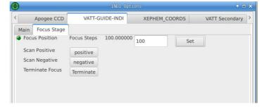
Set focus steps to 100 for tweaking, 1000 or more for defocusing to make collimation setting.
