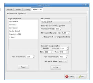
Max RA and DEC duration can also be adjusted from the main PHD2 window (Scope: Mx RA/DEC). A value between 100-150, rather than the Direct Camera value of 2500, works better for on-slit guiding.
