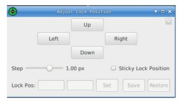
Checking the "Sticky Lock Position" will prevent losing centering if re-calibration is done (automatically) after pressing the PHD button.
