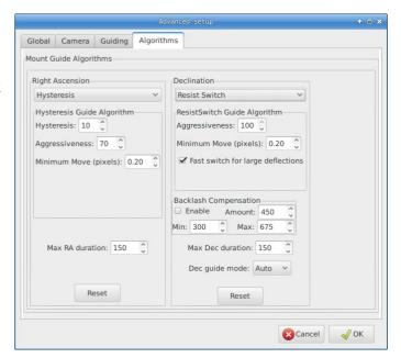
Note the menu options under both RA and Dec, though Hysteresis and Resist Switch are probably the only options needed.
