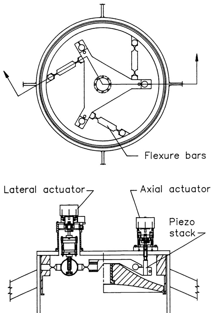
Figure 3: Six axis collimation stage.
