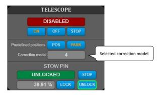
**ON/OFF** button enables/disables the telescope drives.
