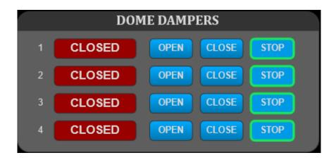
**OPEN** button starts opening the specific dome damper.
