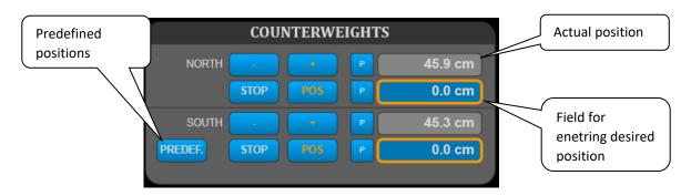
**POS** button moves the counterweight to the desired position.
