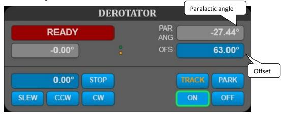
**SLEW** button slews the derotator to the required position.
