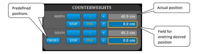
**POS** button moves the counterweight to the desired position.
