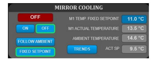
**ON** button starts the mirror cooling system and mirror fans.
