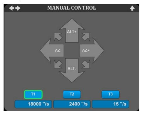
• T1, T2, T3 button selects the speed for manual movement of the telescope.
