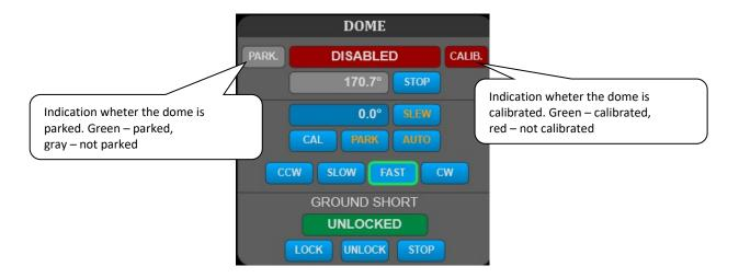
**SLEW** button starts slewing the dome to the inserted position.
