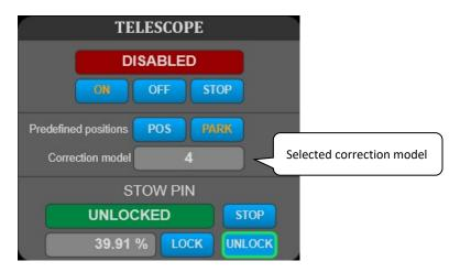
**ON/OFF** button enables/disables the telescope drives.
