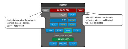
SLEW button starts slewing the dome to the inserted position.
