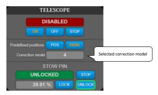
**ON/OFF** button enables/disables the telescope drives.
