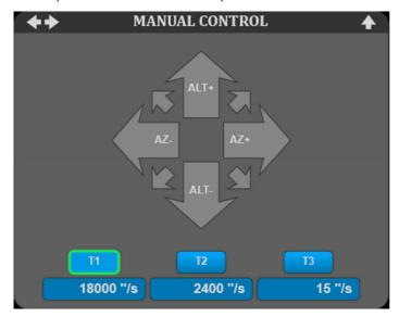
• T1, T2, T3 button selects the speed for manual movement of the telescope.
