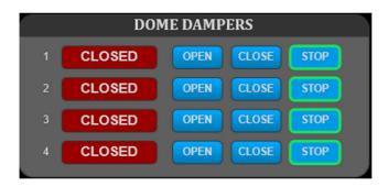
$\ensuremath{\mathbf{OPEN}}$  button starts opening the specific dome damper.
