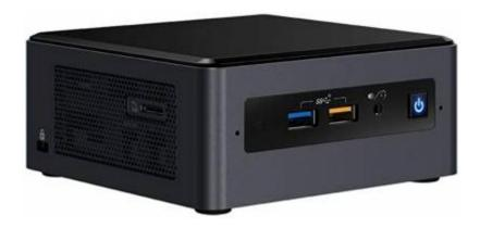
It is an Intel NUC, located on top of the server rack in the instrument room. We call it the sacrificial PC because it is **not** turned off nor disconnected during a lightning shutdown.
