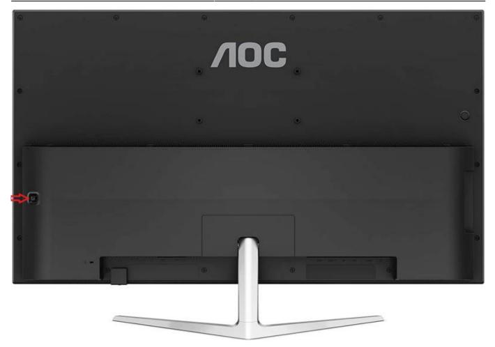
Note the red arrow (left edge of the picture). It points to a multipurpose button. If you hold it down for a couple of seconds, it toggles the monitor on/off. If you touch it briefly, it brings up the monitor menu, and then moving the button up-down-left-right joystick style, allows you to navigate the menu.
