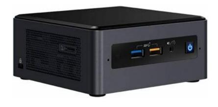
It is an Intel NUC, located on top of the server rack in the instrument room. We call it the *sacrificial* PC because it is **not** turned off nor disconnected during a lightning shutdown.
