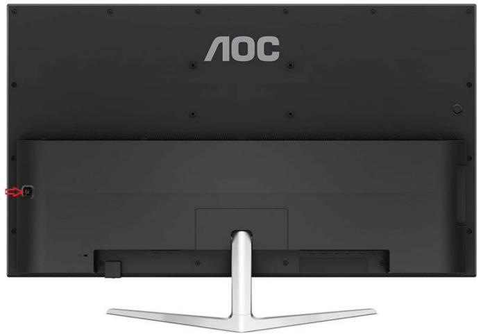
Note the red arrow (left edge of the picture). It points to a multipurpose button. If you hold it down for a couple of seconds, it toggles the monitor on/off. If you touch it briefly, it brings up the monitor menu, and then moving the button up-down-left-right joystick style, allows you to navigate the menu. The AOC 4k monitors are U4308V.
