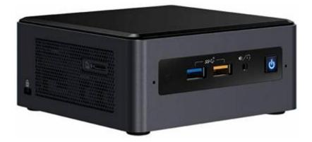
It is an Intel NUC, located on top of the server rack in the instrument room. We call it the *sacrificial* PC because it is **not** turned off nor disconnected during a lightning shutdown.
