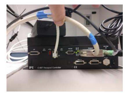
The most important part of this box is the on/off switch located on the bottom right next to the e stop. In lightning shutdown, turn this switch off. When you come back up from lightning shutdown turn this switch on before you turn vatttel on.
