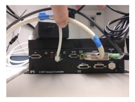
The most important part of this box is the on/off switch located on the bottom right next to the e stop. In lightning shutdown, turn this switch off. When you come back up from lightning shutdown turn this switch on before you turn vattel on.
