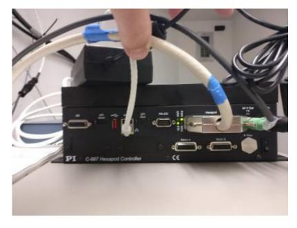
The most important part of this box is the on/off switch located on the bottom right next to the e stop. In lightning shutdown, turn this switch off. When you come back up from lightning shutdown turn this switch on before you turn vatttel on.
