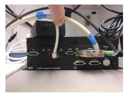
The most important part of this box is the on/off switch located on the bottom right next to the e stop. In lightning shutdown, turn this switch off. When you come back up from lightning shutdown turn this switch on before you turn vattel on.
