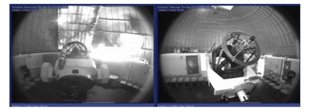
This is the standard "Park" position. At a Declination of -32 degrees, this is 25 degrees from the local horizon and aligns with the Flat Field panel (when the dome is rotated accordingly).
