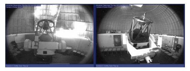
The Celestial equator is approximately 60 degrees above the local horizon when the telescope is at an HA of 0. Thus commanding (0,0) in HA, Declination coordinates results in this position.
