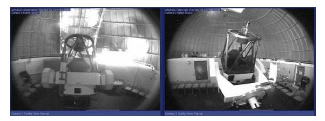
The Celestial equator is approximately 60 degrees above the local horizon when the telescope is at an HA of 0. Thus commanding (0,0) in HA, Declination coordinates results in this position.
