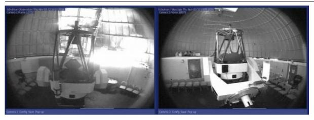
The zenith position is HA,Dec = 0, local latitude. For Mount Lemmon the Declination of the zenith is approximately 32 degrees. Thus the zenith position is a good orientation to verify proper pointing of the telescope. The telescope box and fork arms (bottom edge) should be parallel to the ground. If the fork arms are observed to be rotated slightly there is likely a pointing problem (or a time related issue).
