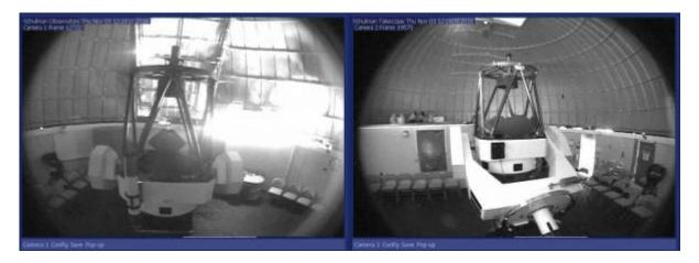
The zenith position is HA,Dec = 0, local latitude. For Mount Lemmon the Declination of the zenith is approximately 32 degrees. Thus the zenith position is a good orientation to verify proper pointing of the telescope. The telescope box and fork arms (bottom edge) should be parallel to the ground. If the fork arms are observed to be rotated slightly there is likely a pointing problem (or a time related
