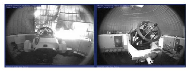
This is the standard "Park" position. At a Declination of -32 degrees, this is 25 degrees from the local horizon and aligns with the Flat Field panel.
