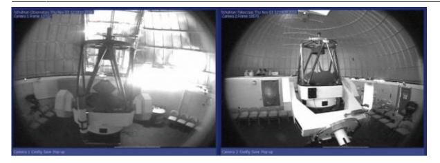
The zenith position is HA,Dec = 0, local latitude. For Mount Lemmon the Declination of the zenith is approximately 32 degrees. Thus the zenith position is a good orientation to verify proper pointing of the telescope. The telescope box and fork arms (bottom edge) should be parallel to the ground. If the fork arms are observed to be rotated slightly there is likely a pointing problem (or a time related issue).
