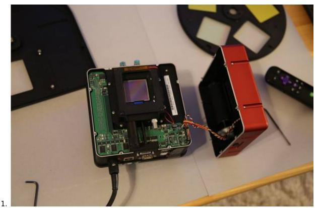
5. The black knurled plug contains the desiccant. Carefully unscrew it from the CCD chamber.
