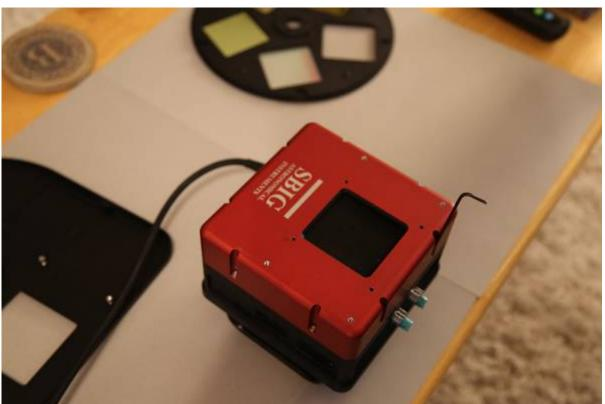
4. Carefully lift the upper portion without unplugging or tugging on the wires that connect to the shutter.
