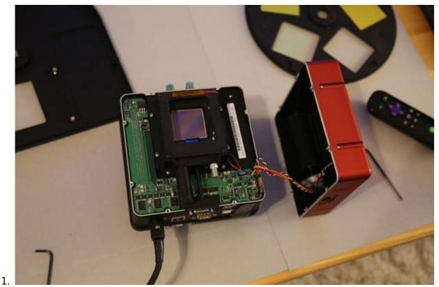
5. The black knurled plug contains the desiccant. Carefully unscrew it from the CCD chamber.
