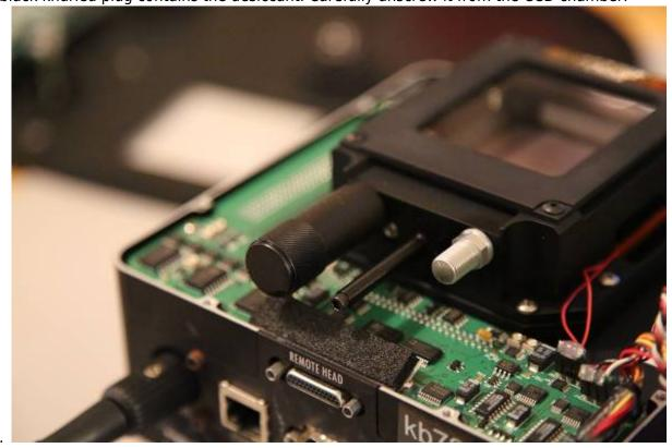
6. Cover the hole to the CCD chamber with a piece of electrical tape while drying the desiccant.
