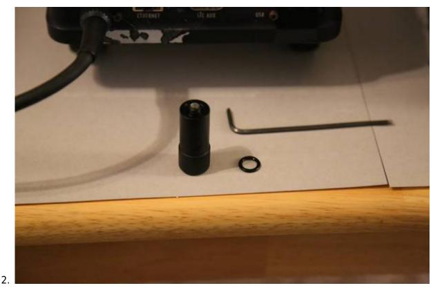
8. Bake plug (without O-ring) in an oven heated to 350F degrees for 4 hours. After baking and once it is cool to the touch, reinstall the plug and reassemble the CCD camera.
