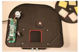
3. Now remove the 8 bolts around the middle of the camera body in order to access the internal parts.
