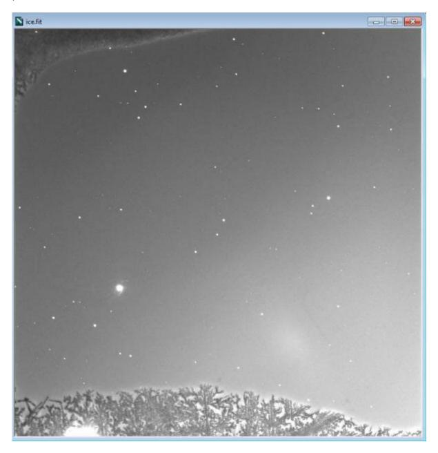
The above clearly shows frost. However, ice usually forms a translucent (foggy) circle that changes size while the chip is cooled (and then is "locked in" once the chip reaches temperature). These are all indications the desiccant needs to be dried out. There is a plug in the camera body that stores the desiccant to be recharged.
