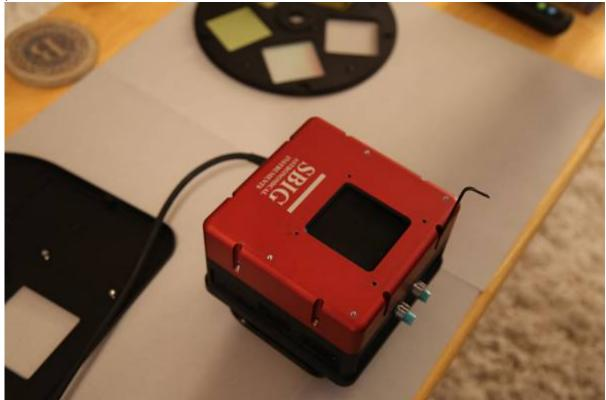
2. Carefully lift the upper portion without unplugging or tugging on the wires that connect to the shutter.
