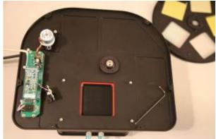
3. Now remove the 8 bolts around the middle of the camera body in order to access the internal
