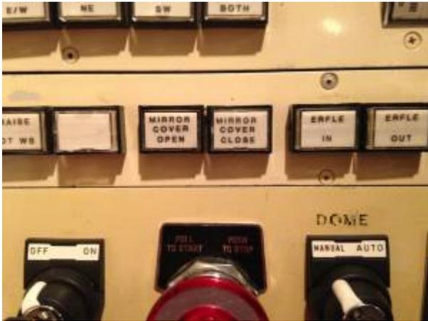
3. Close the dome shutter. Hold button until you are sure shutter is closed. On the weather computer, in the box labeled Telemetry, you will see Dome State in bold. Underneath this, it should read closed. Please double check by looking (with a flashlight if the dome is dark), that the dome really is closed as well.
