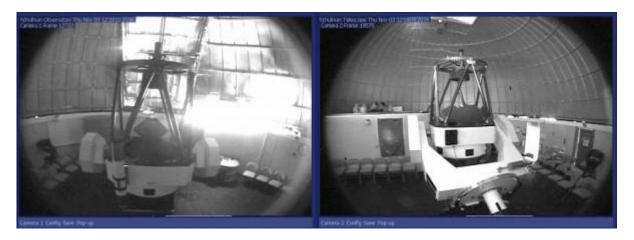
The zenith position is (HA,Dec) = (0, local latitude). For Mount Lemmon the Declination of the zenith is approximately 32 degrees. Thus the zenith position is a good orientation to verify proper pointing of the telescope. The telescope box and fork arms (bottom edge) should be parallel to the ground.
