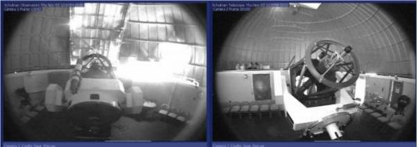
This is the standard "Park" position. At a Declination of -32 degrees, this is 25 degrees from the local horizon and aligns with the Flat Field panel (when the dome is rotated accordingly). Also see the Telescope Limits page for more information.
