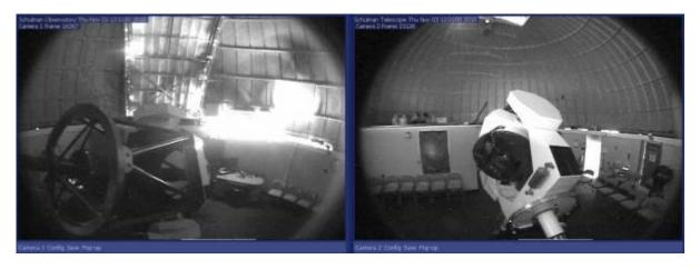
This is the HOME position for the telescope. The telescope may be found in this position for a number of reasons including maintenance, initialization, and potential problems. Nota Bene: This position is at the L1 positive limits for both RA (HA) and Declination axes. This position is fully west to the mechanical limit and fully north to the mechanical limit.
