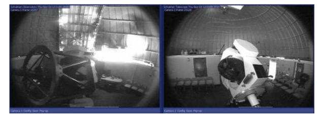
This is the HOME position for the telescope. The telescope may be found in this position for a number of reasons including maintenance, initialization, and potential problems. Nota Bene: This position is at the L1 positive limits for both RA (HA) and Declination axes. This position is fully west to the mechanical limit and fully north to the mechanical limit.
