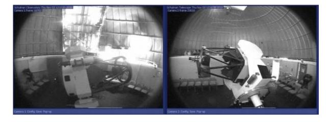
This position (at any Declination) is approximately +5.2 hours in HA. This is the L1 positive limit. The telescope is typically found in this high HA because the tracking was left on. Tracking turns off when the HA limit is reached. There is no potential for damage by reaching this position... but it is VERY poor operator etiquette.
