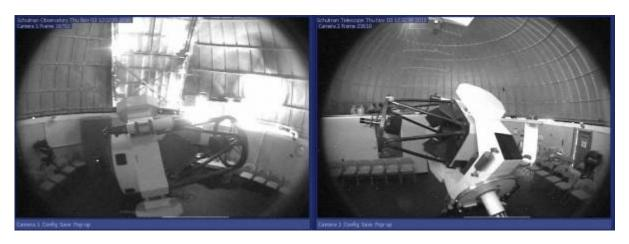
This position (at any Declination) is approximately +5.2 hours in HA. This is the L1 positive limit. The telescope is typically found in this high HA because the tracking was left on. Tracking turns off when the HA limit is reached. There is no potential for damage by reaching this position... but it is VERY poor operator etiquette.
