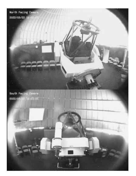
This is the HOME position for the telescope. The telescope may be found in this position for a number of reasons including maintenance, initialization, and potential problems. Nota Bene: This position is at the L1 positive limits for both RA (HA) and Declination axes. This position is fully west to the
