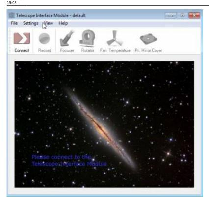
Connect to the TIM unit (by clicking the connect button) and navigate to the "Primary Mirror Cover" tab.
