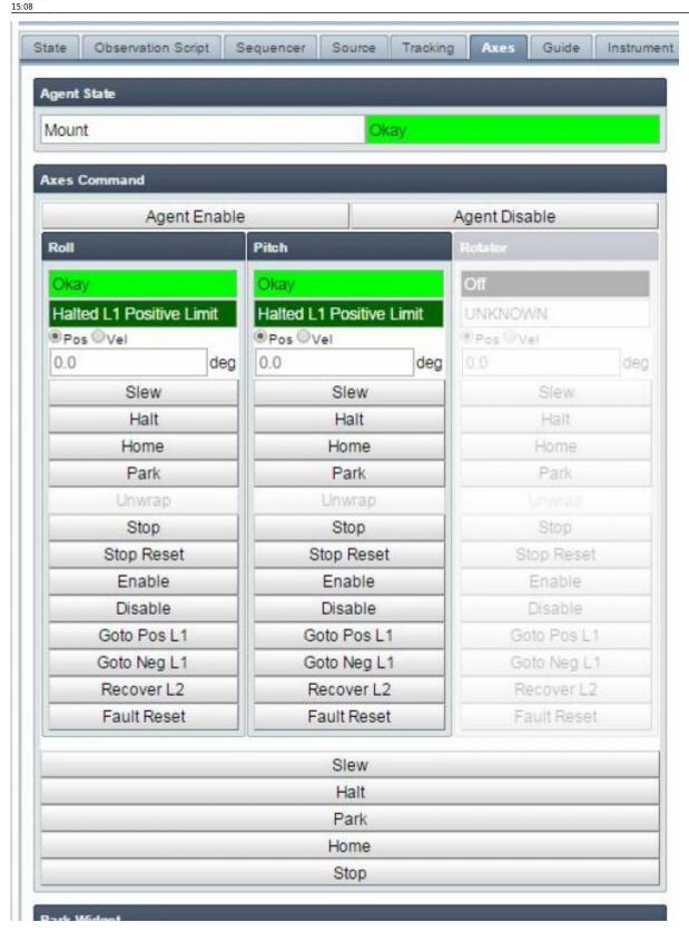
Now go to the *Source* tab and move the telescope out of the limits to a valid sky position. If the telescope is not going to be used immediately, typically the telescope is sent to the Park position. Remember to stop the tracking loop (via the big button or the right that says "Stop Tracking Loop", if observing is not going to start. The Zenith position is inputted in the picture below.
