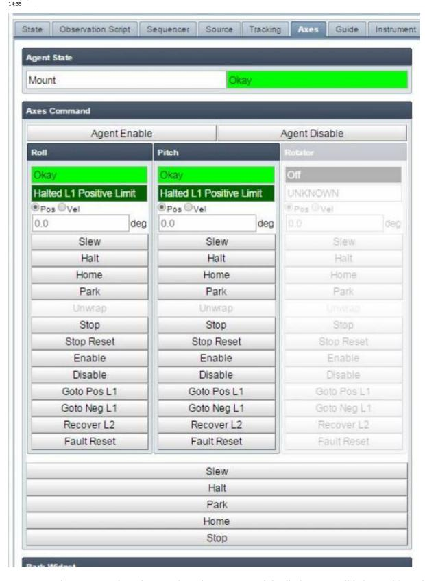
Now go to the *Source* tab and move the telescope out of the limits to a valid sky position. If the telescope is not going to be used immediately typically the telescope is sent to the Park position. Remember to stop the tracking loop if observing is not going to start. The Zenith position is inputted in the picture below.
