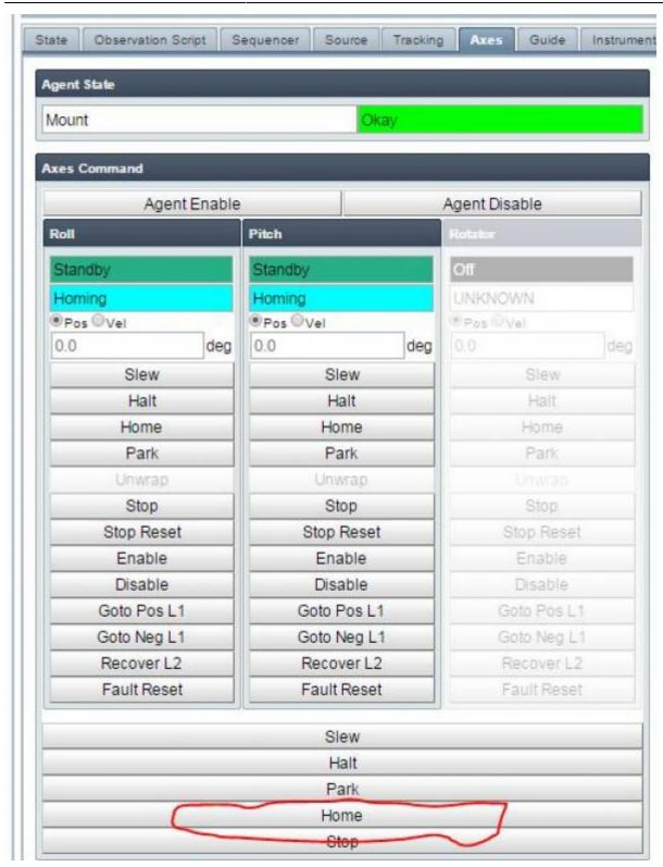
Once homed successfully the state field will briefly go to "stopped" and then finally "L1 Positive Limit" in both axes:
