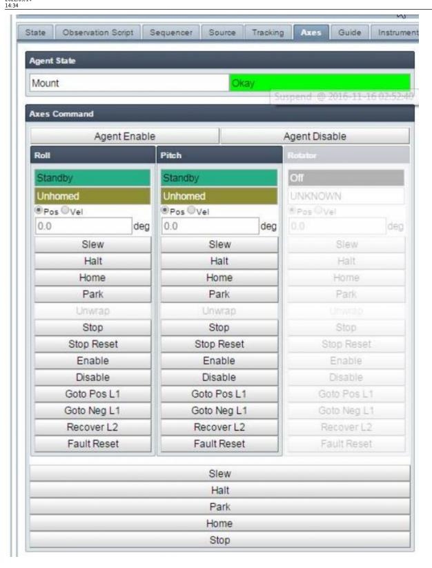
Press the large *HOME* button (circled below) to move both axes simultaneously to the home position. See Telescope Orientation for the correct position.
