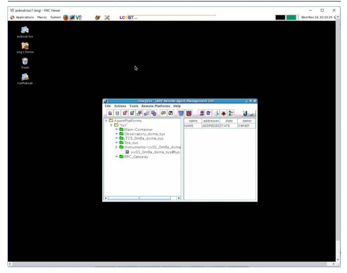
The small icons to the right of processes can be pressed to expand them and reveal the list as shown. Once the "Instruments-xx01\_0m8a\_doma" process is loaded under its section PubSub is ready to communicate with the telescope (and the user). The "RPC\_Gateway" process will not show up until communication to PubSub through the web browser commences. This is in the next step. It is OK to close the VNC window.
