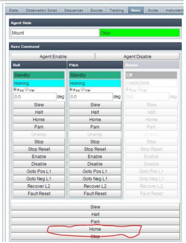
3. Once homed successfully the state field will briefly go to "stopped" and then finally "L1 Positive Limit" in both axes:
