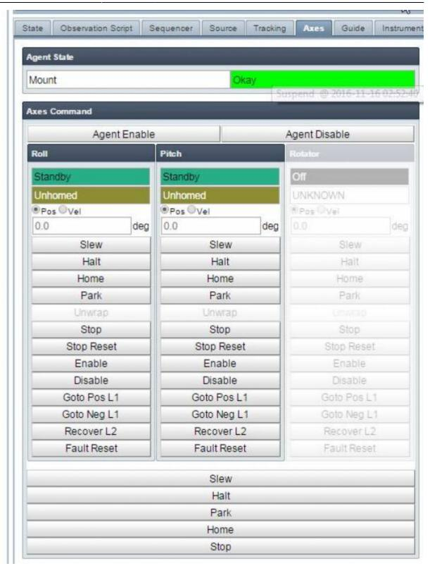
2. Press the large *HOME* button (circled below) to move both axes simultaneously to the home position. See Telescope Orientation for the correct position.
