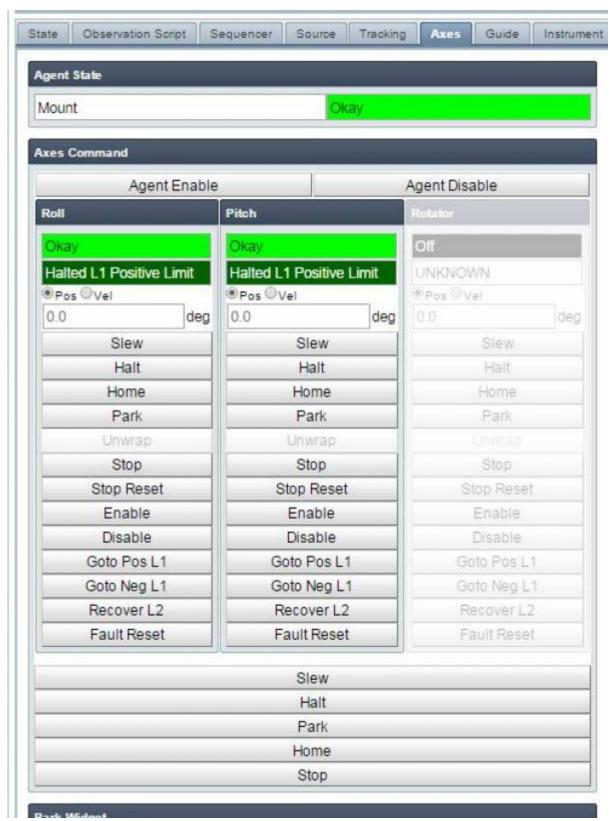
4. Now go to the *Source* tab and move the telescope out of the limits to a valid sky position. If the telescope is not going to be used immediately typically the telescope is sent to the park position. Remember to stop the tracking loop if observing is not going to start. The zenith position is inputted in the picture below.
