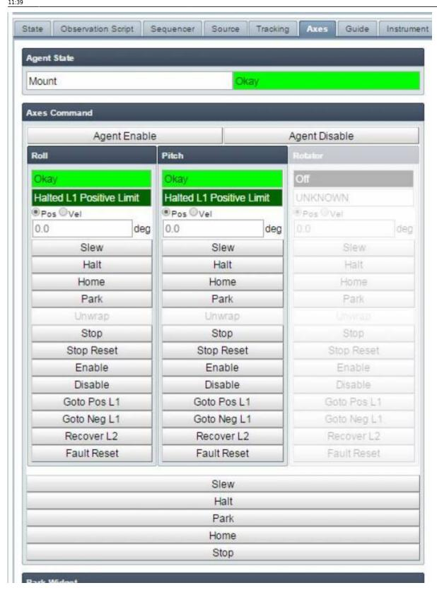
Now go to the *Source* tab and move the telescope out of the limits to a valid sky position. If the telescope is not going to be used immediately, typically the telescope is sent to the <u>Park</u> position. Remember to stop the tracking loop (via the big button or the right that says "Stop Tracking Loop", if observing is not going to start. The <u>Zenith</u> position is inputted in the picture below.
