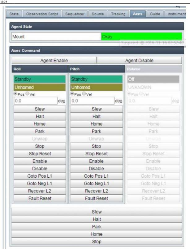
Press the large *HOME* button (circled below) at the bottom of the window to move both axes simultaneously to the home position. See <u>Telescope</u> Orientation for the correct position.
