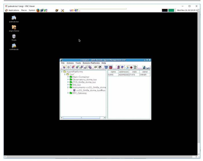
The small icons to the left of each folder icon can be pressed to expand them and reveal the list as shown. Once the "Instruments-xx01\_0m8a\_doma" process is loaded under its section, PubSub is ready to communicate with the telescope (and the user). The "RPC\_Gateway" process will not show up until communication to PubSub commences through the web browser. This is in the next step. It is OK to close the VNC window.
