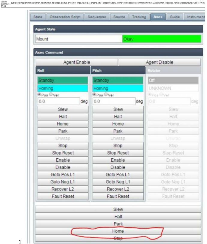
3. Once homed successfully the state field will briefly go to "stopped" and then finally "L1 Positive Limit" in both axes:
