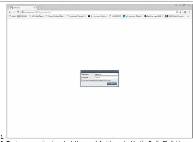
2. The log on name is unimportant. However *default* is required for the Config File field. 3. Press the "OK" button to continue.
