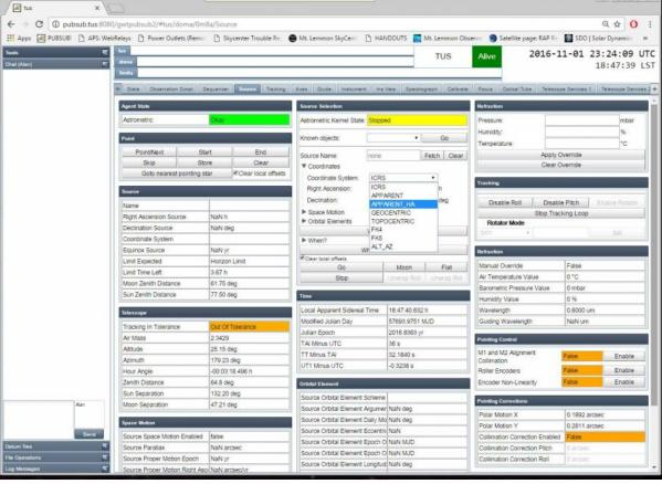
10. Now input an Hour Angle and Declination that corresponds to the desired position. Shown below is the input for Zenith. Press the "GO" button that is below the coordinate systems to move the
