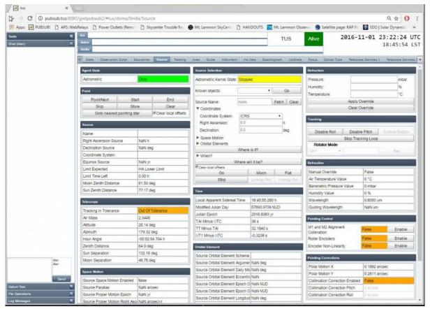
9. Under the "Coordinate System" select "Apparent HA." This is typically the engineering method for moving the telescope to particular positions. "Alt\_AZ" (Altitude, Azimuth) is another. Please read the section on Astronomical Coordinates Review for more information on the range of values for this coordinate systems.
