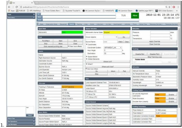
11. Once the telescope reaches the desired position it will be tracking at the sidereal rate. Note that "Astrometric Kernal State" is green and reads "Tracking." In addition the "Tracking Tolerance" field reads "In Tolerance."
