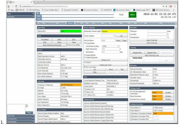
2. The "Astrometric Kernal" reads "Stopped" and the "Tracking Tolerance" field reads "Out of Tolerance."
