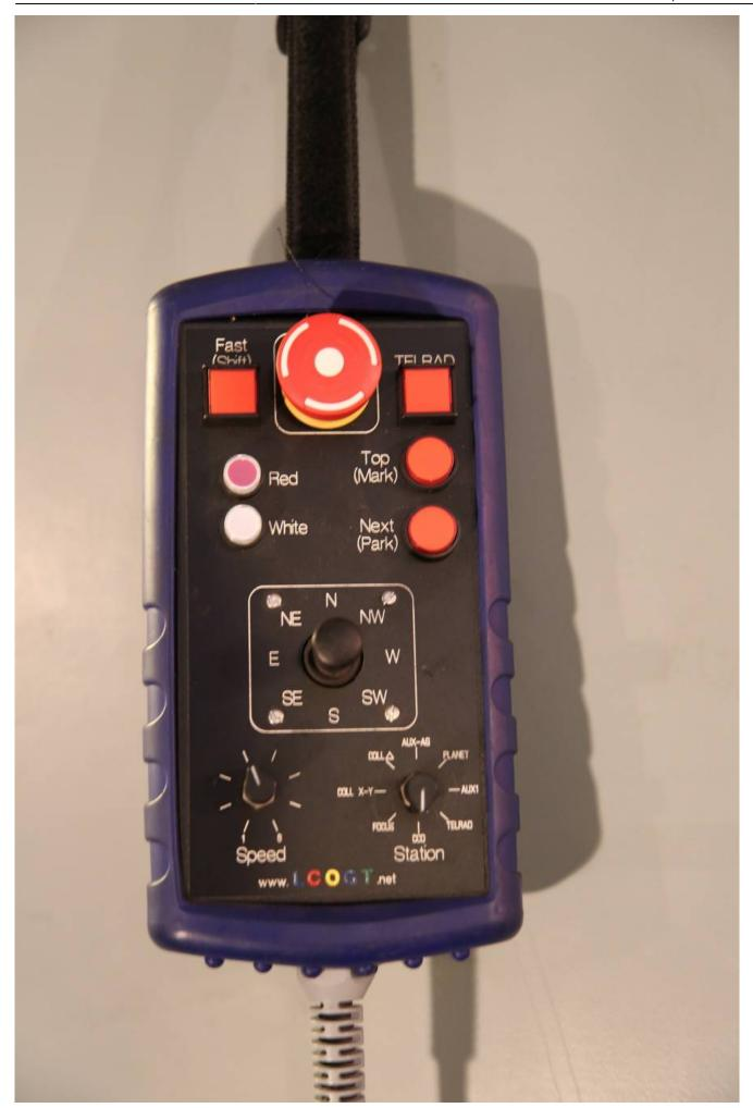
• The Red button at the top of the paddle is an Emergency Stop (E-Stop) plunger. Pressing this button will de-energize the brakes (causing them to clamp down) and disconnect the drives
