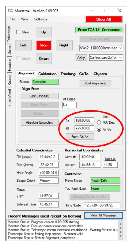
Click the Home Seek in the Alignment tab and then confirm align home by clicking "yes". The telescope with quickly move west and north a bit and then slowly continue north and east until it hits its home switches. If it does not find the switches it will time out with a warning the the messages field.
