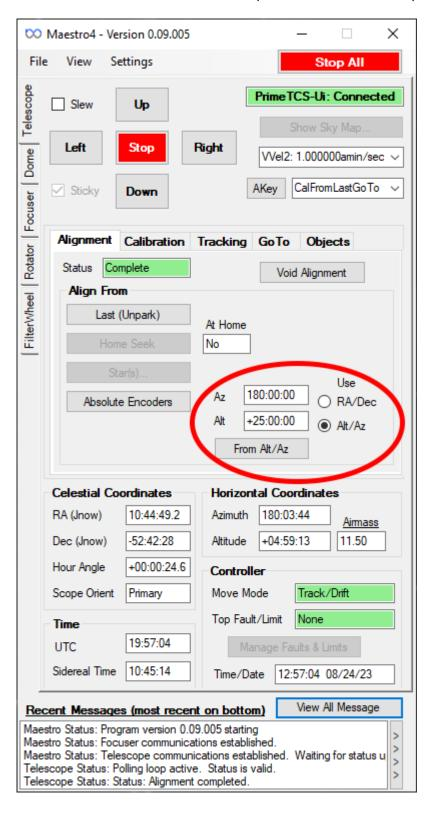
Click the Home Seek in the Alignment tab and then confirm align home by clicking "yes". The telescope with quickly move west and north a bit and then slowly continue north and east until it hits
