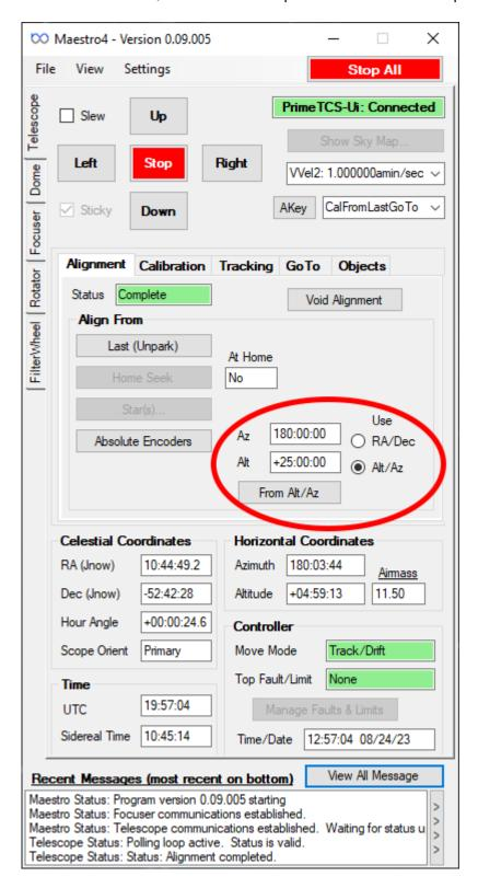
Click the Home Seek in the Alignment tab and then confirm align home by clicking "yes". The telescope with quickly move west and north a bit and then slowly continue north and east until it hits its home switches. If it does not find the switches it will time out with a warning the the messages field.
