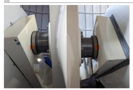
Once placed in this position make sure the telescope isn't moving on its own away from that point. If it does it is too far out of balance. Easiest solution is to put it in a balanced configuration. If you are too impatient to do this at this moment you can have a friend do their best impression of Atlas until the Controller is turned on and the drives begin holding the telescope in position.
