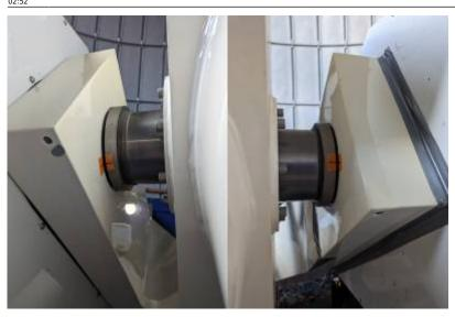
Once placed in this position make sure the telescope isn't moving on its own away from that point. If it does it is too far out of balance. Easiest solution is to put it in a balanced configuration. If you are too impatient to do this at this moment you can have a friend do their best impression of Atlas until the Controller is turned on and the drives begin holding the telescope in position.
