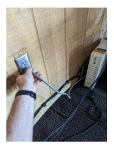
Next you must turn on the UPD. Press and hold the corresponding "on" button for at least a second until you hear a beep, then let go. the UPS will immediately supply power to their output plugs, so no further button pressing is necessary on the UPS. Last update: 2023/08/23 public:catalinas:lemmon:phillips\_24:startup\_procedure https://lavinia.as.arizona.edu/~tscopewiki/doku.php?id=public:catalinas:lemmon:phillips\_24:startup\_procedure&rev=1692821448 13:10
