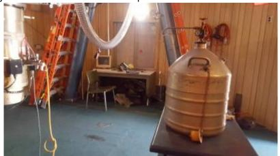
2. Hook up yellow rubber hose to LN2 tank. It should already be hooked to the instrument, but if not hook up to the LN2 fill port.
