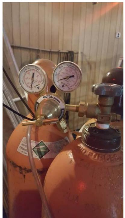
8. Watch the LN2 dewar very carefully, and adjust the gold handle on the N2 as needed so the pressure read out on the LN2 dewar maintains at 9 psi. Note in the picture below it's reading at ~5 psi.
