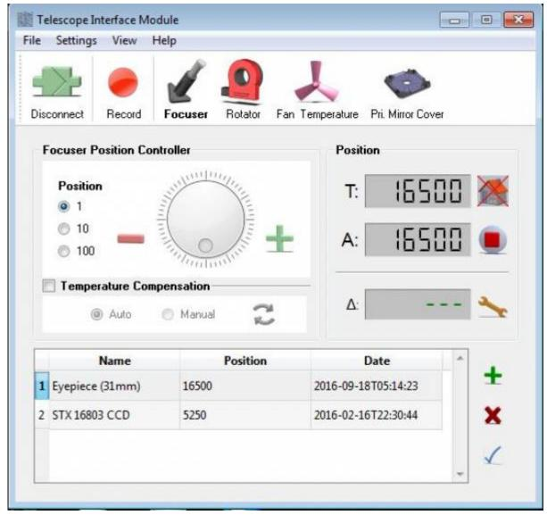
If not at eyepiece value, select this position and press the blue check mark.
