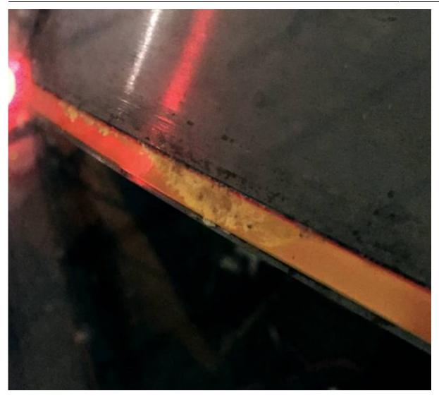
If the blots are large enough or partially obscure the optical tape a drive fault may be triggered (see the smeared moth remains above). The drives might receive
